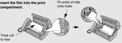
7 Rotate the front gear as shown until the film is taut.
